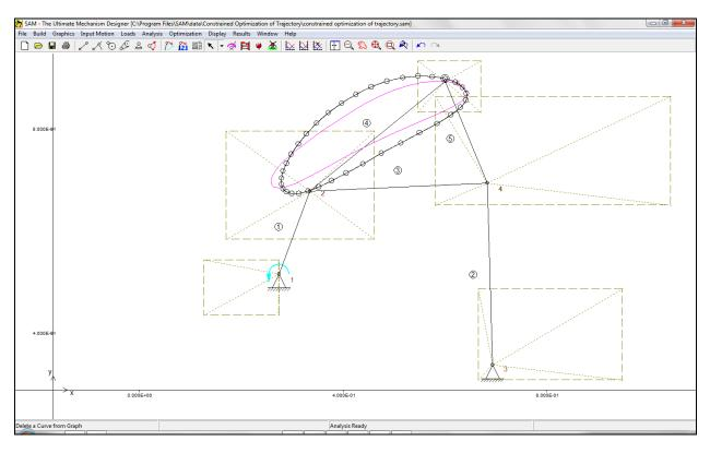
As one can see, node 1 is on the edge of the parameter rectangle, which suggests that better solutions might be possible if that limit is relaxed. The easiest way to relax all parameter space limits, without effecting the constraint defined by the penalty value, is to modify the Simplex settings (see below)
